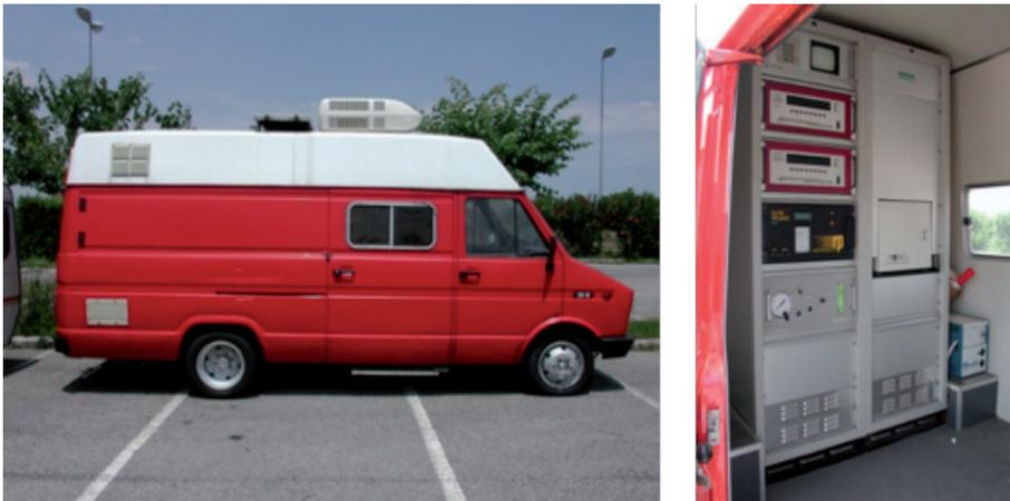
Figure 3. Mobile laboratory equipped with automatic analyzers in compliance with EPA standards.
