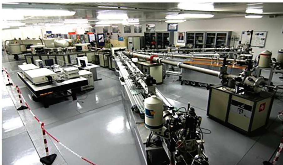
Figure 1. The AMS-IBA system at the CEDAD - University of Salento. 6 beamlines and 4 ion sources are connected to the Tandetron accelerator for radiocarbon dating and compositional analysis of materials
