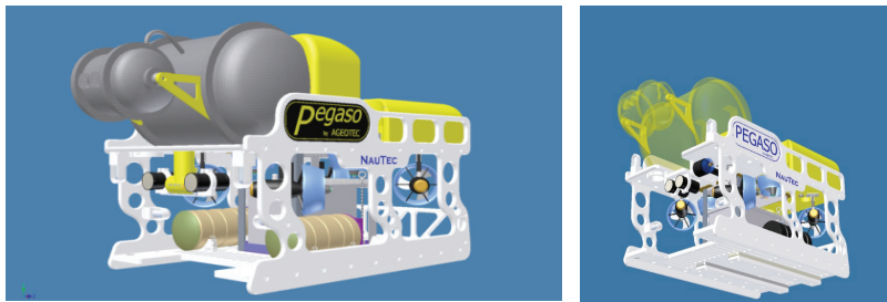
Figure 3. concept of ROV with Pegasus configuration that can accommodate the UTR
