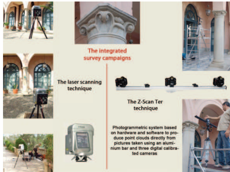
Figure 6. The integrated survey campaign for acquisition of the complex geometry of a capital in the Utveggio Castle's portico. A comparison between the time-of-flight laser scanning technique and the Z-Scan photogrammetric technique (Graphic design by Francesco Di Paola).
