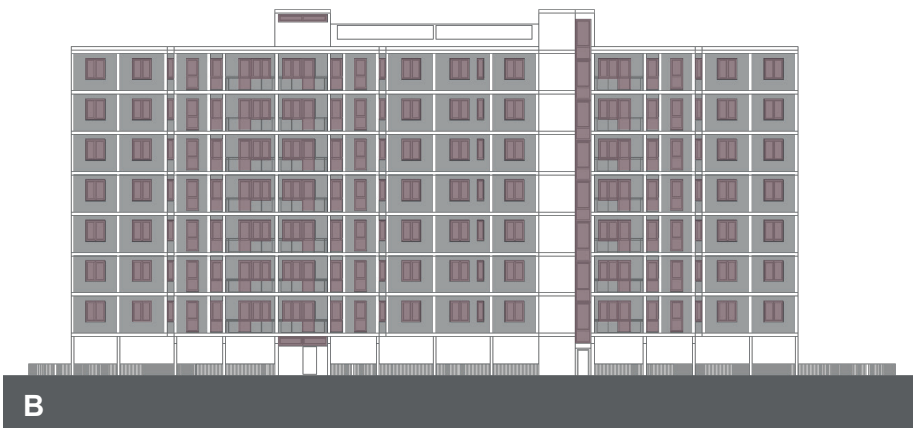
Figure 3. A) A façade as a system: modular rhythm, joints, and panel logic derived from an analytical abacus extracted from a digital model. B) Same façade elevation with window openings highlighted (fenestration pattern), extracted from the digital model, to make the modular rhythm and openings' hierarchy legible. Credits: Vannini, C. 2025
