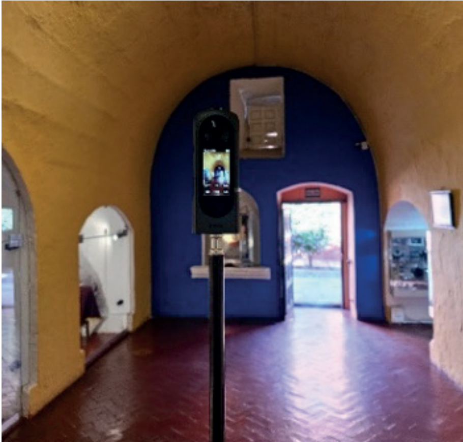
Figure 4. 360° spherical camera positioned at one of the scanning stations inside the community infirmary dormitory, illustrating the data acquisition setup used during the three-dimensional documentation process.
