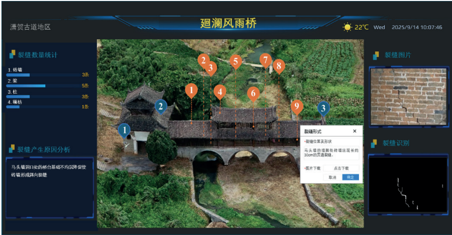
Figure 8. Visualization platform for apparent crack detection of the wind-rain bridge.
