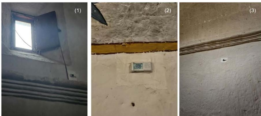
Figure 2. Placement of sensors in the study spaces. (1) Sensor 1 placed in Cell A at a height of 3.20 m; (2) Sensor 7 placed in Cell D at a height of 2.45 m; (3) Sensor 5 placed in Cell B at a height of 3.50 m.
