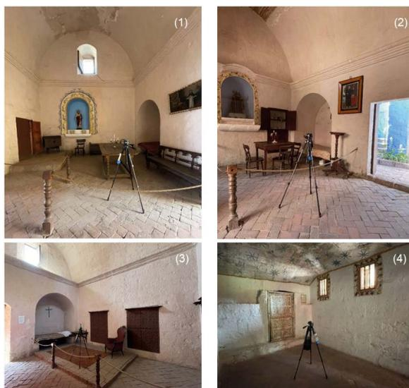
*Figure 9. Lux Meter placement in interior spaces, mounted on tripod at 0.70 m height; (1) position of equipment in Cell A; (2) position of equipment in Cell B; (3) position of equipment in Cell C; (4) position of equipment in Cell D.*
