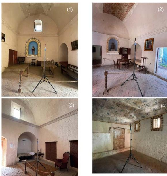
*Figure 10. Sound Level Meter placement in interior spaces, mounted on tripod at 1.80 m height. (1) position of equipment in Cell A; (2) position of equipment in Cell C; (3) position of equipment in Cell D; (4) position of equipment in Cell D.*
