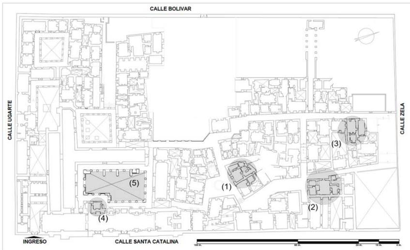
*Figure 1. Location of the study areas on the base plan of the Santa Catalina Monastery in Arequipa. (1) Cell A; (2) Cell B; (3) Cell C; (4) Cell D; and (5) Main Cloister.*
