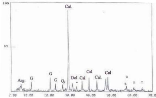
Figure 3. X-ray diffraction patterns of sample 1-1.
