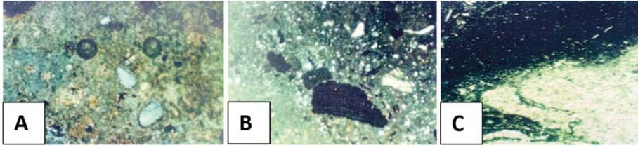
Figure 7. Petrography of samples. Image A shows the microscopic observation of the intermediate plaster located between the main (external) plaster and the mortar. Image B presents the microscopic observation of the coating, while image C shows the microscopic observation of the masonry stone.
