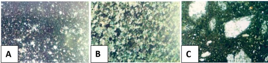
Figure 8. Petrography of samples. Image A shows the microscopic observation of the masonry stone. Image B presents the microscopic observation of the transformation of this rock from its original form into a microcrystalline limestone, while image C shows the microscopic observation of the plaster.
