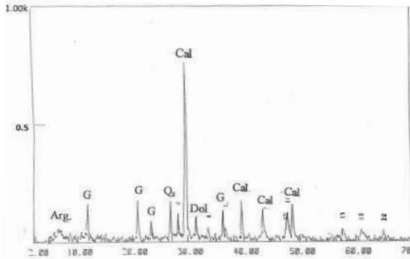
Figure 4. X-ray diffraction patterns of the sample 1-2.
