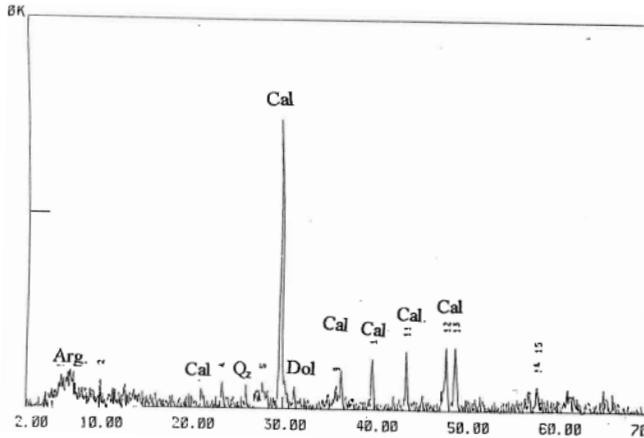
Figure 5. X-ray diffraction patterns of sample 2.
