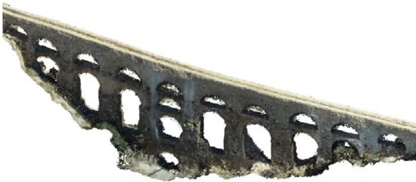
Figure 6. Point cloud imported into Autodesk Revit.
